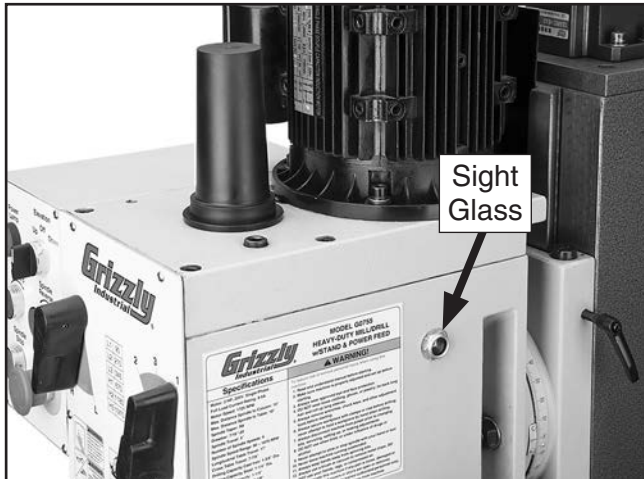
Figure 42. Headstock sight glass.
